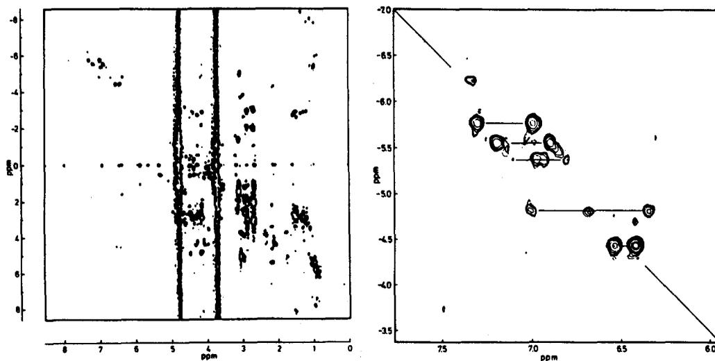
FIG. 11. Left: complete DQ  $^1\text{H}$  spectrum of porcine adenylate kinase at 360 MHz. Right: aromatic part of the DQ spectrum (connectivities indicated).
