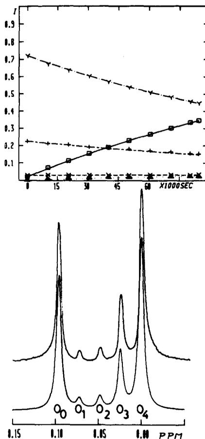
FIG. 19. Top: Time course of the concentration of five different  $^{18}\text{O}$  species of inorganic phosphate in a reaction mixture consisting of: 0.2 mM ADP/100 mM  $\text{PO}_4$  ( $^{18}\text{O}$  enrichment 90% at  $t=0$ ) /0.18 mM S1 1 mM  $\text{MgCl}_2$ . Bottom: Spectrum of inorganic phosphate after 23.5 hr reaction time in the reaction mixture as above. Upper spectrum: experiment. Lower spectrum: Computer fit as described in the text (Rösch *et al.*<sup>(120)</sup>).
