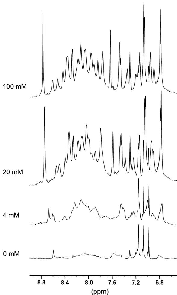
**Fig. 3.**  $^1\text{H-NMR}$  titration of Vpr(13–33) with dodecyl-*PCho*. 1D proton spectra of 2.2 mM Vpr(13–33) peptide at 298 K without dodecyl-*PCho* (bottom) and with increasing concentrations of dodecyl-*PCho* (shown on left hand side). Shown is the region of aromatic and amide protons.
